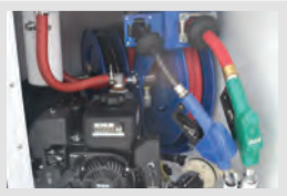
Inside Box with 40 GPM Electric Start Gas Engine
