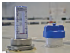
DEF Gauge and Fill Cap
